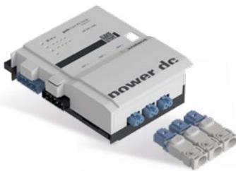
The 24 VDC; 30W power supply unit with flat surface mounted housing which can be fitted on DIN rails for decentralized installation can be added to the system. It receives mains from the upstream module and forwards mains and bus supply to the following modules. The output is wired parallel to three 2-pole connectors.
