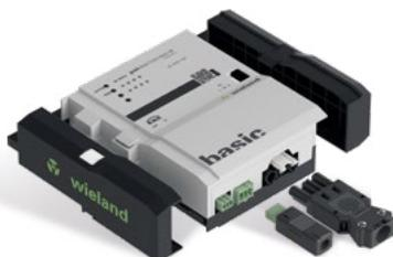
The 1-phase supplied KNX base module with flat surface mounted housing, which can be fitted on DIN rails for decentralized installation, supports 6 extension modules. They support all the common inputs and outputs, and they provide extensive room automation with only one physical address. The manual operation level allows function tests without prior system integration. The electrical connections, which are pluggable in accordance with IEC 61535, separate automation and installation.
