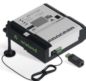
The bidirectional gateway for 32 channels is an independent KNX unit in a flat surface-mounted housing, which can be mounted on DIN rails for decentralized installation. The gateway is based on the EnOcean Equipment Profiles (EEP). In addition to the software for commissioning, there is comfortable manual operation available via a display. The ETS application also has an extensive logic/control range. The KNX connection is pluggable.
