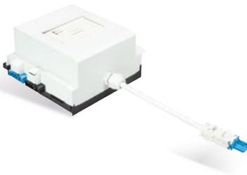
The power supply is used to supply 24 V DC consumers, the surface mounted housing can be fitted on DIN rails for decentralized installation. It is not suitable as a KNX power supply. The module receives its power supply from an upstream gesis® FLEX module. All electrical connections are pluggable according to IEC 61535.
