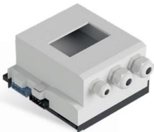
The REG module for DIN rail surface mounting for decentralized installation can be used to install DIN rail mounted devices according to DIN 43880 with up to four module widths. Mains and bus supply are passed from upstream to downstream module. Mains supply can be tapped internally. Depending on the model, a clear cover to protect the internal device is mounted, cable glands already integrated or must be provided on site.
