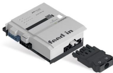
The intermediate feed with flat surface mounted housing, which can be fitted on DIN rails for decentralized installation, allows a mains supply separate from the base module within a modular system. This means that the output loads can be split over different fuse circuits. It can be integrated in the system as often as required. The electrical connections, which are pluggable in accordance with IEC 61535, separate automation and installation.
